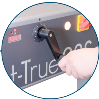
Manual Back Gauge Adjustment Fine-tune control for precision cutting
